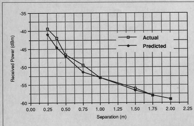
Figure 2. Predicted vs. actual Ku band link performance.
