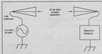
Figure 1. Test set up to determine actual vs. far field boundary.
