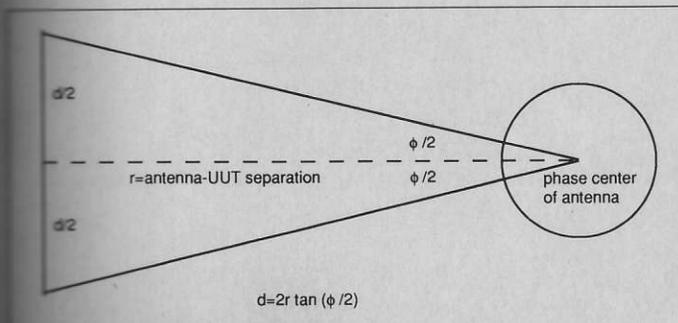
Figure 4. Illuminated Spot Diameter.
