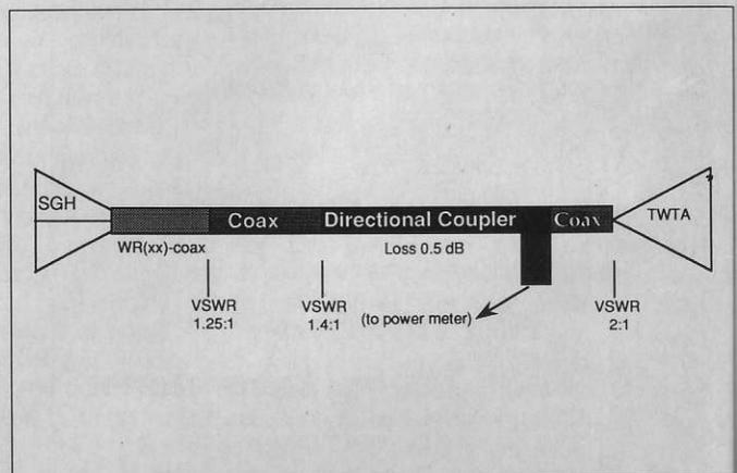
Figure 3. Example calculation of power loss budget.
