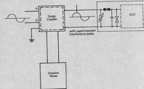
Haefely is renowned worldwide as a manufacturer of quality Impulse Test Systems. The **PC 6-288 combination wave tester**, simulates lightning transients in accordance with **IEC 801-5/D, IEEE 587.1, C62.41, SAE-AE4L, ABD0013 and ABD0007** and other industrial and aerospace standards. The **modular design** enables the use of different waveshaping plug-ins and an RS 232 computer interface.
