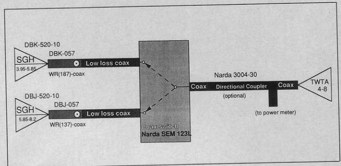
Figure 6. Test Set Up, 3.95 GHz to 8.2 GHz.
