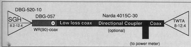
Figure 7. Test Set Up, 8 GHz to 12.4 GHz.
