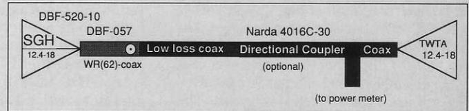
Figure 8. Test Set Up, 12.4 GHz to 18 GHz.
