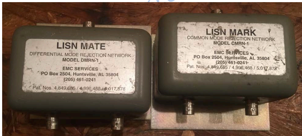
Figure 10: The author's well-worn collection of EMC Services LISNMATE (DMRN) and LISNMARK (CMRN) mode separators. At this writing these are not commercially available.
