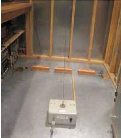
**Figure 7a.** “Reality” check configuration. Separation of radiating line from back wall the same as when on table-top ground plane.
