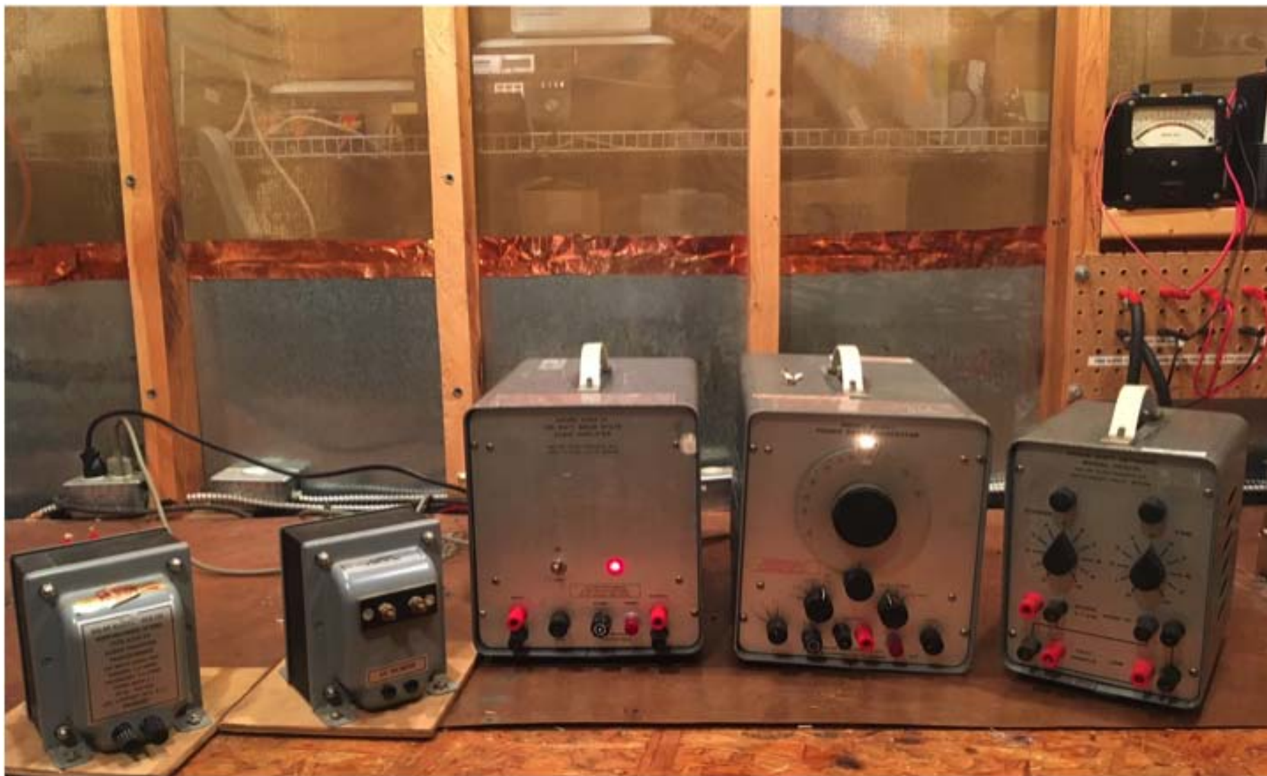
Figure 7: Solar Electronics test equipment specifically designed for CS01. All equipment shown is still valid and useful for CS101, except the phase-shift network on the right.
