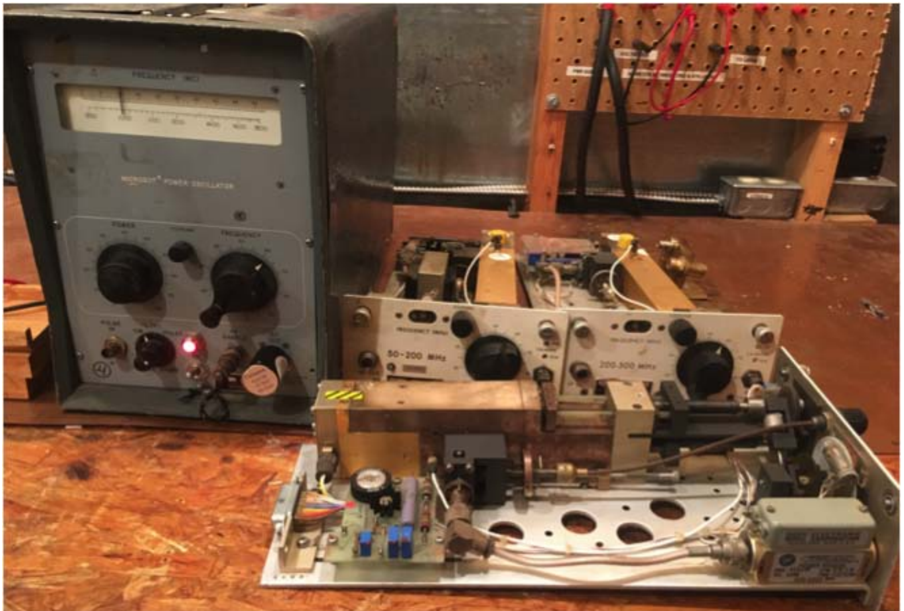
Figure 6: Susceptibility signal sources using cavity-tuned oscillators, mainframe and separate plug-ins. Plug-ins show that tuning and coupling was all done mechanically. At the end of a long day of CS02 and RS03, the technician's hands were callused and cramped.
