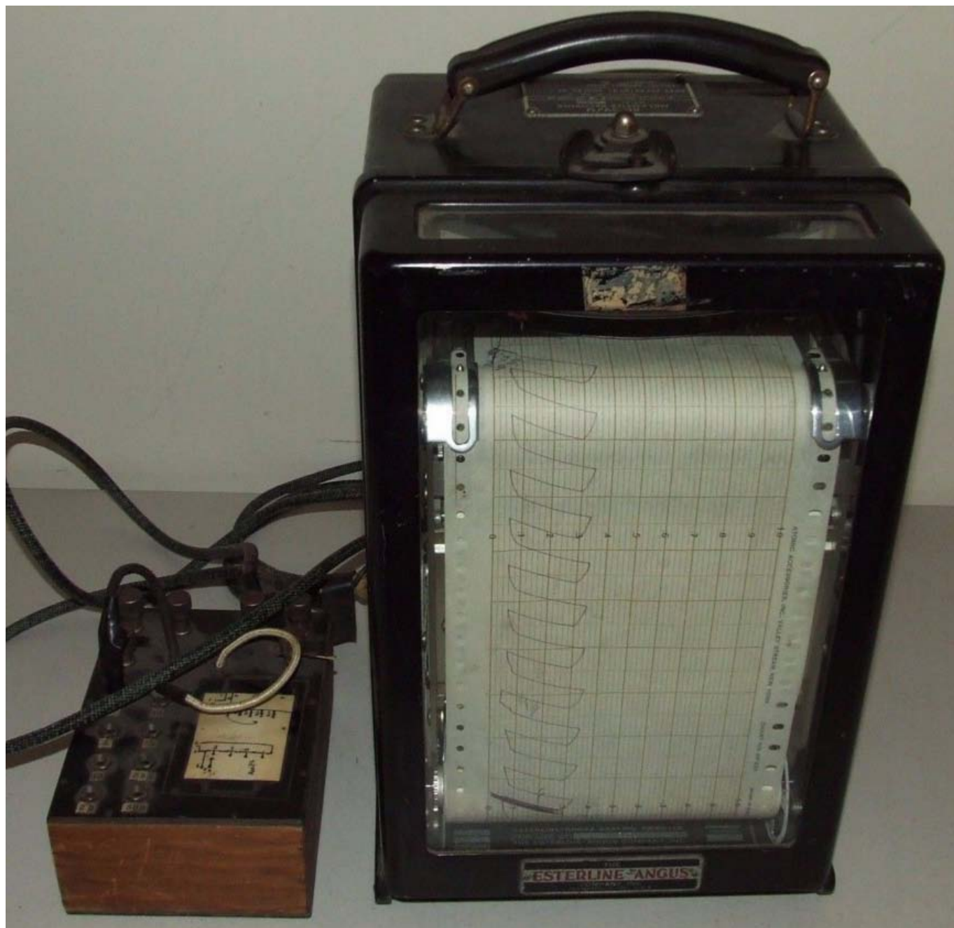
Figure 5: Stoddart chart recorder to be used with Figure 1 receivers to generate plotted data.
