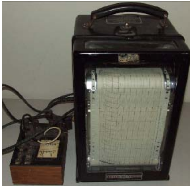
Figure 5: Stoddart chart recorder to be used with Figure 1 receivers to generate plotted data.
