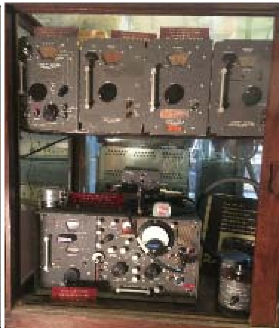
Figure 2: Empire Devices NF-105 manually tuned receiver with plug-ins, 1950s – 60s.
