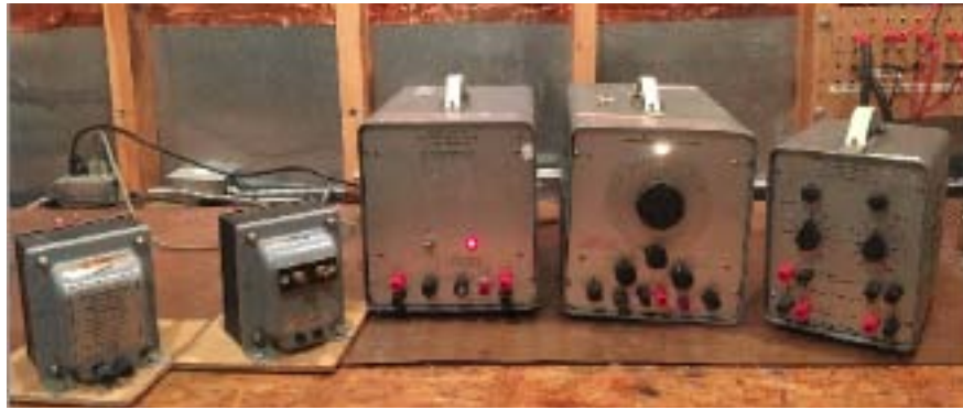
Figure 7: Solar Electronics test equipment specifically designed for CS01. All equipment shown is still valid and useful for CS101, except the phase-shift network on the right. 39
