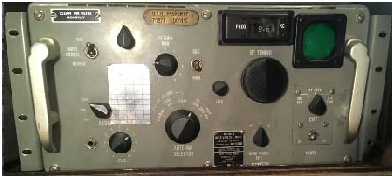
Figure 3: AN/BRR-3, Polaris class submarine vlf receiver. Polaris class submarines carried sea-launched, nuclear-tipped ballistic missiles. The AN/BRR-3 received instructions to launch Armageddon.
