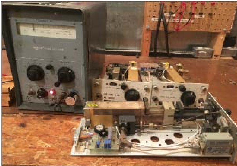
Figure 6: Susceptibility signal sources using cavity-tuned oscillators, mainframe and separate plug-ins. Plug-ins show that tuning and coupling was all done mechanically. At the end of a long day of CS02 and RS03, the technician’s hands were callused and cramped.
