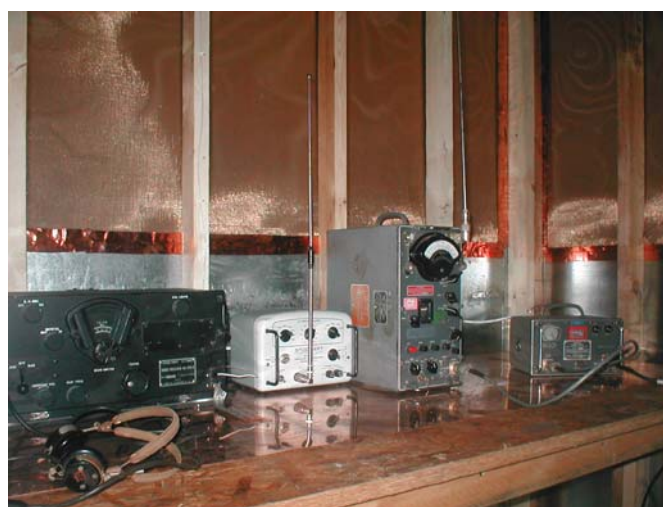
Photographic Plate 1: Re-enactment of NADC-EL-5515 set up that measured the response of an aircraft radio of the period, and used that susceptibility to build a radiated emission limit for MIL-I-6181B in the early 1950s. From left to right: BC-348Q aircraft LW-MW-SW radio, impulse (noise) generator, Stoddart Aircraft Radio Company NM-20 / AN/PRM-1EMI receiver, EMI receiver power supply. (Photo courtesy of EMC Compliance and the Museum of EMC Antiquities).
